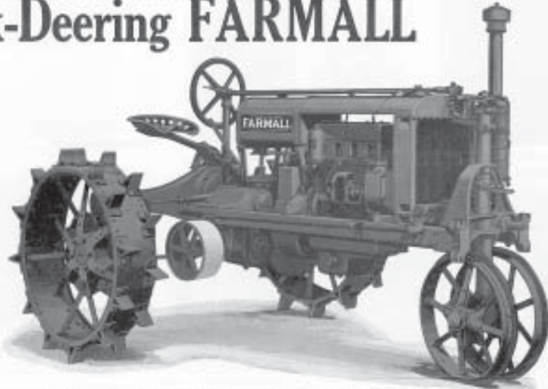
Illustr. 1. This is the two-plow FARMALL—the tractor that is putting agriculture on a new and far more profitable basis. The wheels may be the 22 x 42-inch with spade legs as shown, or 8 x 40-inch with angle legs. Wheel equipment must be specified.
